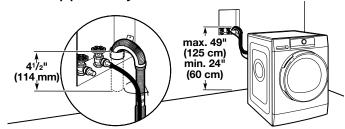
See requirements for floor standpipe drain system.
