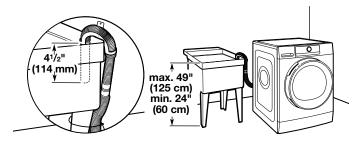
Minimum capacity: 20 gal. (76 L). Top of laundry tub must be at least 24" (60 cm) above floor; install no higher than 49" (125 cm) from bottom of washer.
