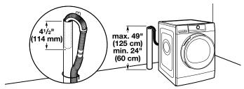
Minimum diameter for a standpipe drain: 2" (51 mm). Minimum carryaway capacity: 17 gal. (64 L) per minute. A 1/4" (6 mm) diameter to 1" (25 mm) diameter Standpipe Adapter Kit is available (Part Number 3363920). Top of standpipe must be at least 24" (60 cm) high; install no higher than 49" (125 cm) from bottom of washer. If you have an overhead sewer and need to pump higher than 96 inches, a sump pump and associated hardware are needed. See "Alternate Parts."
