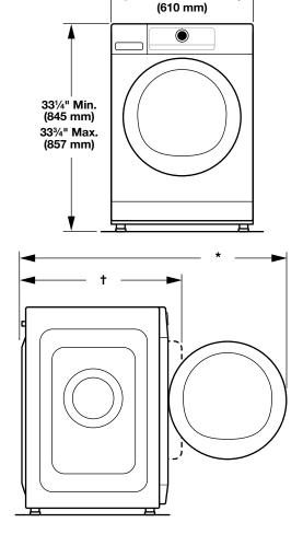
\*2.3 cu. ft. models: 42<sup>15</sup>/16" (1091 mm) 1.9 cu. ft. models: 41<sup>5</sup>/8" (1057 mm)
